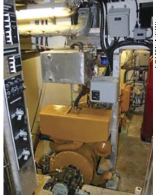
The 275-hp Caterpillar 3406 main on Twin Disc 5114 (3.5:1) marine gear provide 10.5 knots top speed at 1850 rpm. At nine knots (1500 rpm) fuel consumption is approximately five Imp. gals/hour. Fuel capacity is approximately 1450 Imp. gals. There is a 9 kW Kubota genset.
